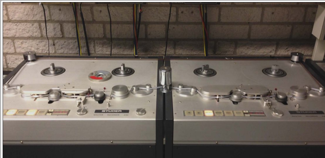
Figure 3: The tape loop setup using the two Studer tape machines in BEA 5. Photo taken by the author.
